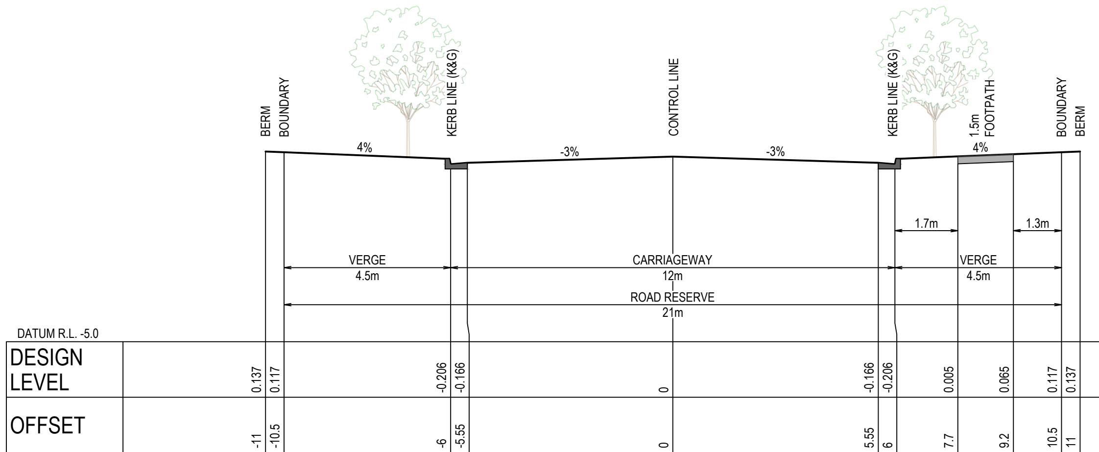
ROAD TYPE 3 - PRIMARY COLLECTOR (12m WIDE PER LOCHINVAR U.R.A. DCP) SCALE 1:100 NATURAL
